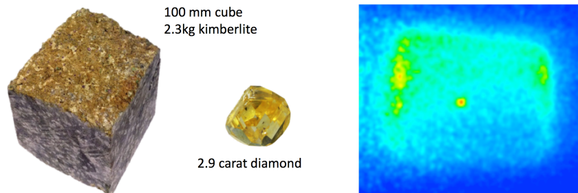
Figure 2. MinPET discovery image for a 2.9 carat diamond buried in the middle of cube of kimberlite of side 100 mm (2.3 kg).
