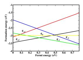
**Figure 4.** Plot of formation energy as a function of the Fermi energy for (a) Mo<sub>Ge</sub>.
