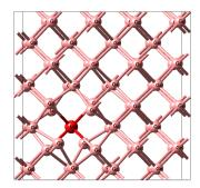
Figure 2. Fully relaxed geometric structures of  $V_{\rm Ge}Mo_{\rm Ge}$  for the N1 configuration.
