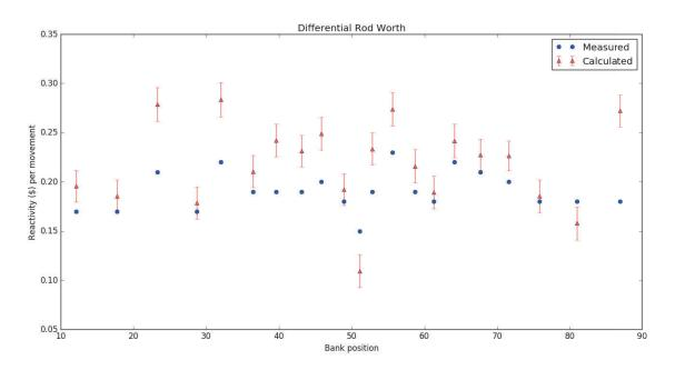
**Figure 2:** A comparison between the calculated and measured differential rod worth curves for control rod 5 calibration
