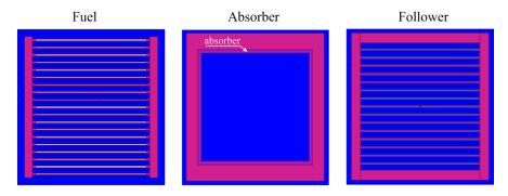
Figure 2: View of the fuel element, absorber and fuel follower
