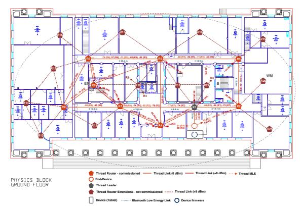
**Figure 2:** Experimental development of Thread network.
