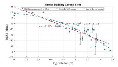
Figure 1: RSSI versus  $log_{10}(d)$  at Tx = 0 dBm.
