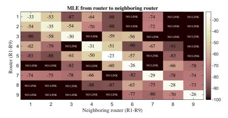
**Figure 3:** Mesh Link Establishment (MLE) by RSS at Tx = +8 dBm.
