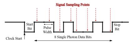
**Figure 2.** Asynchronous transmission begins with a Start bit which serves as the synchronisation indicator. The pulse width of each bit is agreed upon before the transmission begins and the receiver is able to measure the 8 data bits following the Start bit. The Stop bit indicates that the data has stopped, pending the transmission of another Start bit.
