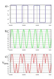
Figure 3. Diagram a) shows the modulating signal which represents the information to be transmitted over the public channel. The carrier signal, shown in b), is a sinusoidal radio signal which will be used for synchronisation. The modulated signal  $V_{BPSK}$ , shown in c), carries general binary data through the public channel.
