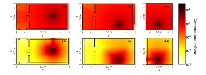
Figure 2. Combined neutron and photon dose maps for the (a) unshielded and (b) shielded geometries, as centred on the generator, i.e. the highest dose regions. The x-y plane is parallel to the floor and the z-axis is in the vertical direction. Solid lines indicate concrete walls, and the dashed region in (ai), (aii) and (bi), (bii) relates to the highest risk accessible area. Any regions with doses above  $10^{-2}$  mSv per hour are considered unsafe for 100 operating hours per year.
