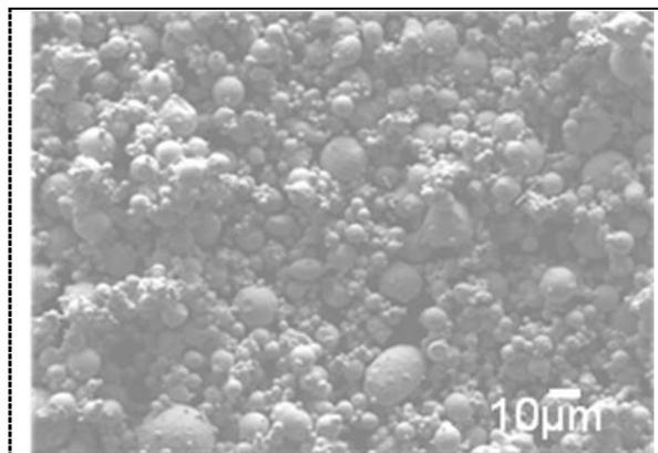
**Figure 1.** SEM micrograph of 2507 stainless steel powder
