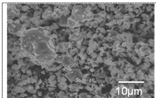
**Figure 2.** SEM micrograph of TiC powder
