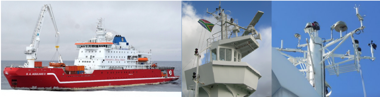
Figure 4: The SA Agulhas II polar research vessel, pictured at Akta Bukta in Antarctica in February of 2015, is equipped with a NovAtel GISTM receiver in the Crow's Nest. The grey dome antenna is located at the very top of the mast, providing an unobstructed view of the sky.
