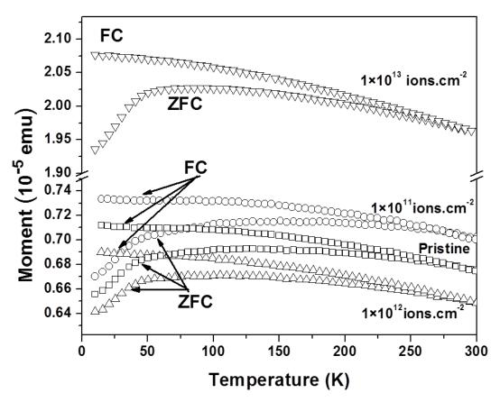
**Figure 2.** Magnetization as a function of temperature of pristine and irradiated  $Ti_{0.95}Co_{0.05}O_{2-\delta}$  thin films deposited at 10 mTorr oxygen partial pressure on LaAlO<sub>3</sub> substrate.
