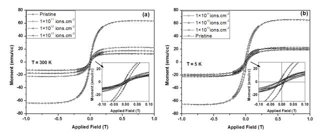
**Figure 3.** *M-H* plots for the pristine and irradiated  $Ti_{0.95}Co_{0.05}O_{2-\delta}$  thin films deposited at 10 mTorr oxygen partial pressure on LaAlO<sub>3</sub> substrate and measured at temperatures: (a) 300 K and (b) 5 K. The insets show the zoomed view of the hysteresis loops in low field region.
