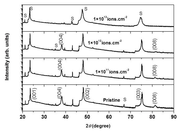
**Figure 1.** XRD pattern of pristine and irradiated  $Ti_{0.95}Co_{0.05}O_{2-\delta}$  thin films deposited at 10 mTorr oxygen partial pressure on LaAlO<sub>3</sub> substrate. The fluence used is indicated in each panel. 'S' denotes the reflections related to LaAlO<sub>3</sub> substrate.
