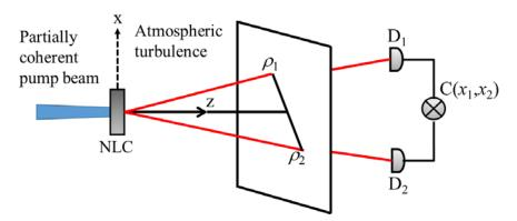
**Figure 1.** Schematic setup that could be used to study the influence of atmospheric turbulence on the coincidence counts. The bump beam is partially spatially coherent.
