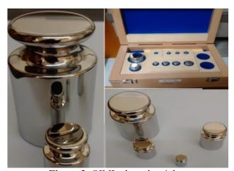
Figure 2: OIML-shaped weights.
