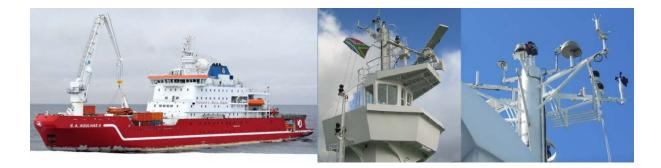
**Figure 4:** The SA Agulhas II polar research vessel, pictured at Akta Bukta in Antarctica in February of 2015, is equipped with a NovAtel GISMT receiver in the Crow's Nest. The grey dome antenna is located at the very top of the mast, providing an unobstructed view of the sky.
