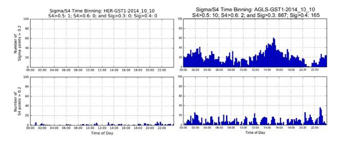
**Figure 6:** Histogram of  $S_4$  and  $\sigma_{\phi} \geq 0.2$  counts recorded on 10 October 2014 at Hermanus (left) and on board the SA Agulhas II (right). Time is in UT.
