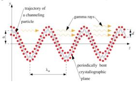
Figure 1: A charged particle captured in a undulating crystal channel [6].
