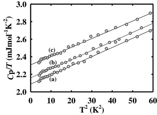
**Figure 3:** Graphs of  $C_p(T)/T$  vs.  $T^2$  plotted for three typical  $(\text{Cr}_{100-x}\text{Al}_x)_{95}\text{Mo}_5$  alloy examples at low temperatures: (a) an ISDW alloy with  $x = 1.0$ , (b) a CSDW alloy with  $x = 6.1$  and (c) a PM alloy with  $x = 2.8$  at.% Al. The solid lines through the data points represent least-square linear fits. The experimental error in  $C_p(T)/T$  is about 1%.
