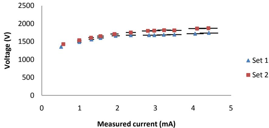
**Figure 3.** Preliminary electrical data: Current into the thruster was measured against the potential difference between the plate and the ring.
