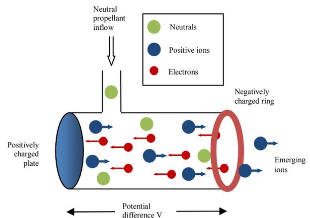
**Figure 1.** Schematic of miniaturised Hall Effect type thruster
