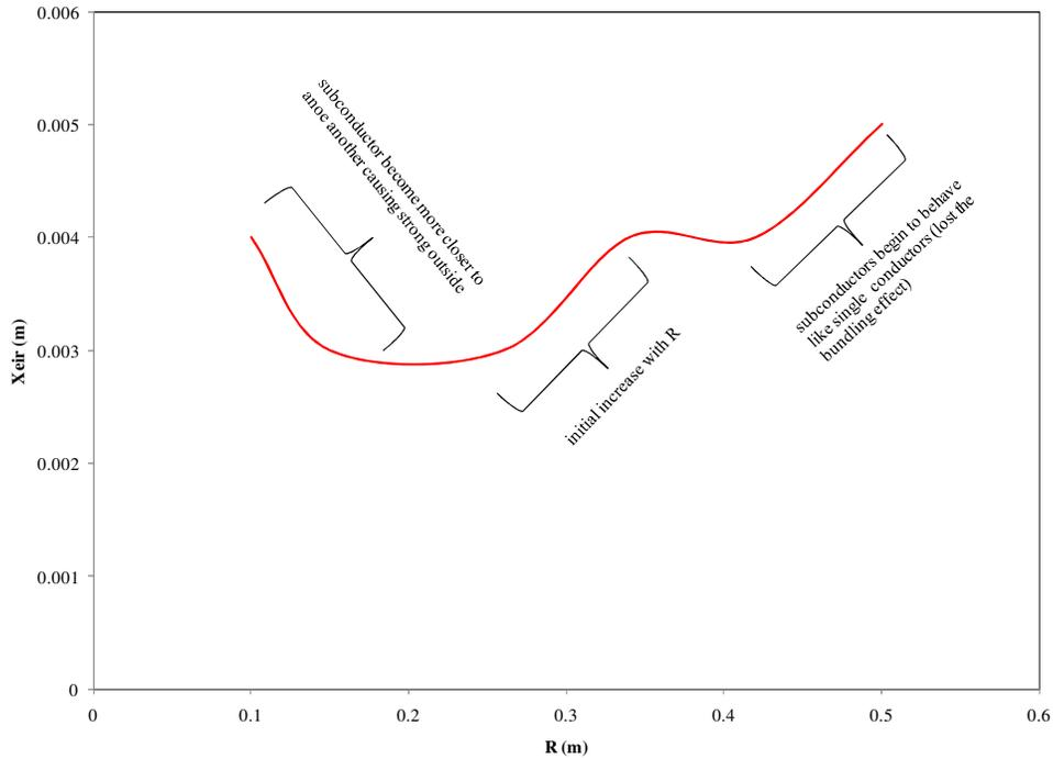
**Figure 6.** Plot of  $x_{eir}$  vs.  $R$  for a four bundle.
