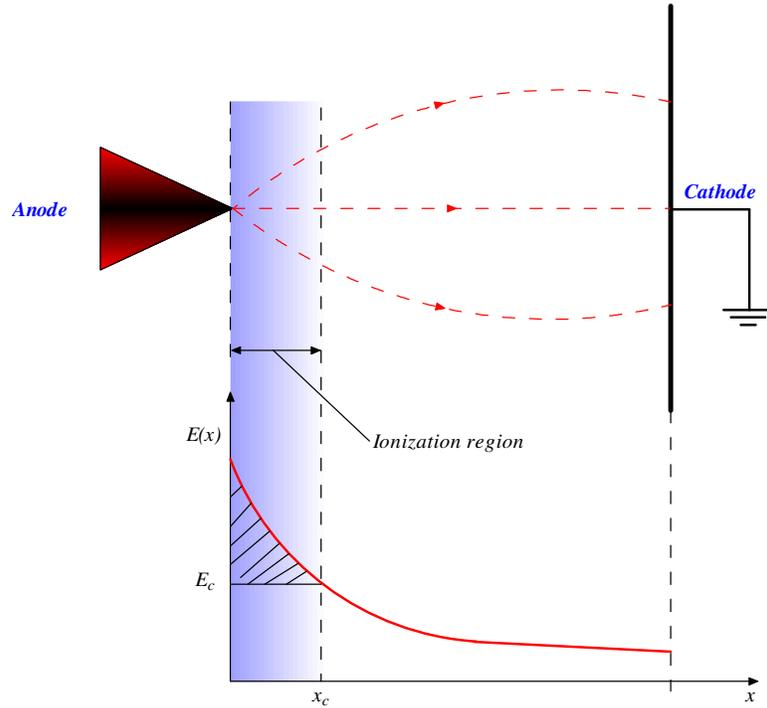
**Figure 1.** Electric field distribution in a non uniform point plane gap [1].
