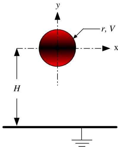
**Figure 2a.** Simulation geometry for single conductor system.
