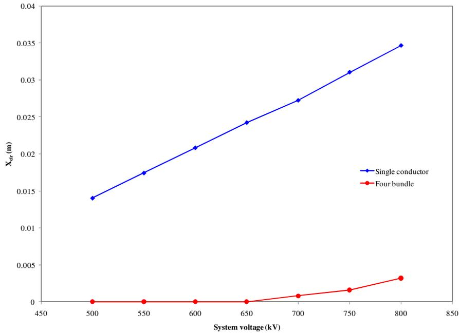
**Figure 3.** Plot of  $x_{eir}$  vs.  $V$  for a single conductor and a four bundle.
