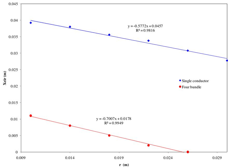
**Figure 5.** Plot of  $x_{eir}$  vs.  $r$  for a single conductor and a four bundle.
