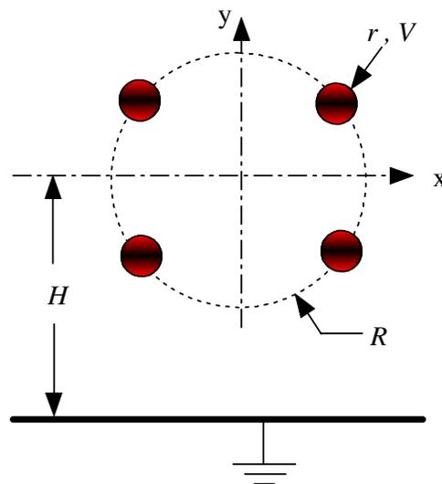
**Figure 2b.** Simulation geometry for a four bundle system.
