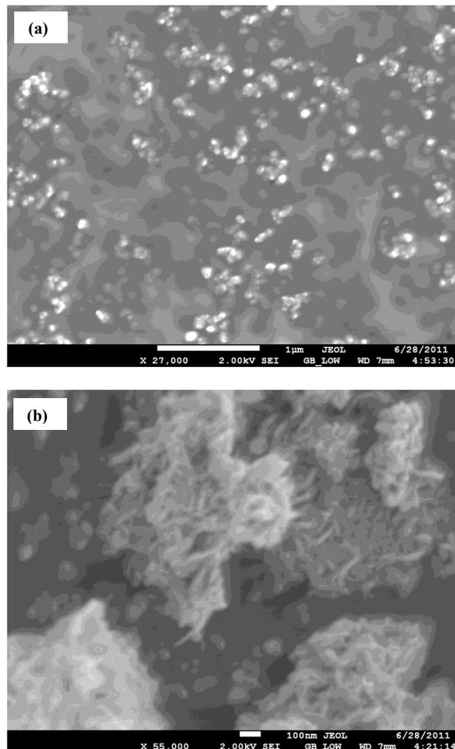
Figure 2: SEM images of ZnO (a) Nanoparticles and (b) clustered Nanorods
