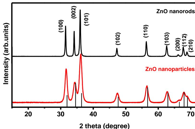
Figure 1: XRD patterns of ZnO nanorods, nanoparticles and standard JPCDS match (card no 80-007)
