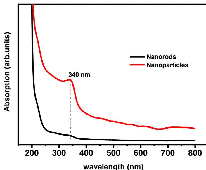
Figure 2: Absorption spectra of both colloidal ZnO nanorods and nanoparticles
