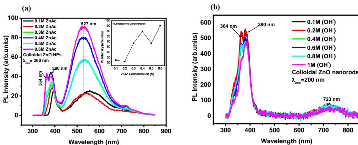
Figure 4: The PL spectra of colloidal (a) ZnO nanoparticles, the inset shows the PL intensity vs concentration of zinc acetate, (b) ZnO nanorods.
