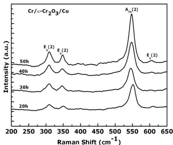
**Figure 1.** The Raman spectra of Cr/ $\alpha$ -Cr<sub>2</sub>O<sub>3</sub> monodispersed spherical core-shell particles
