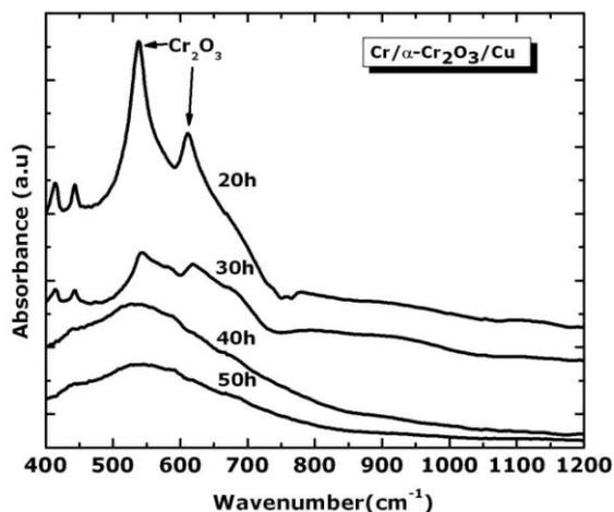
**Figure 2.** The Attenuated Total Reflection spectra for Cr/ $\alpha$ -Cr<sub>2</sub>O<sub>3</sub> monodisperse spherical core-shell particles
