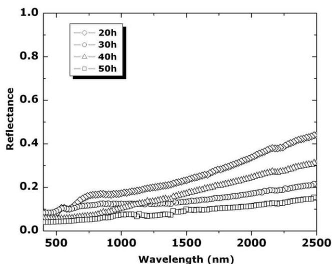
**Figure 5.** The total diffuse reflectance of different samples over the UV-VIS-NIR range.
