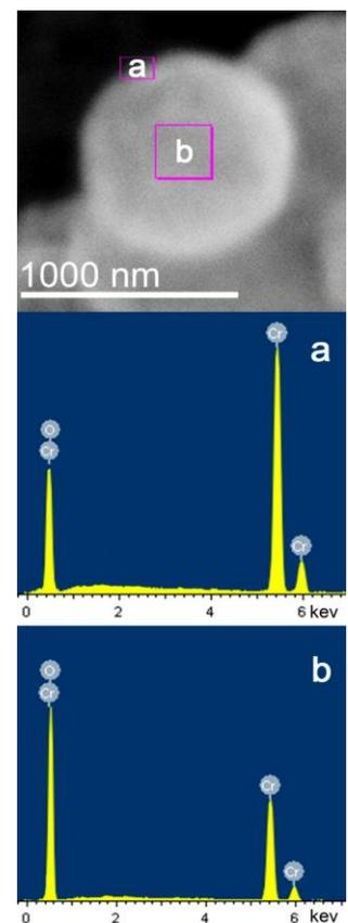
**Figure 4.** Investigation of shell and core of one Cr/ $\alpha$ -Cr<sub>2</sub>O<sub>3</sub> monodispersed particle
