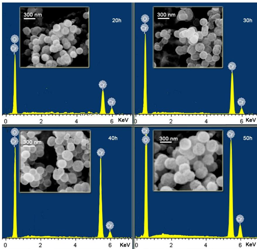
**Figure 3.** SEM/EDS of Cr/ $\alpha$ -Cr<sub>2</sub>O<sub>3</sub> monodispersed spherical core-shell particles
