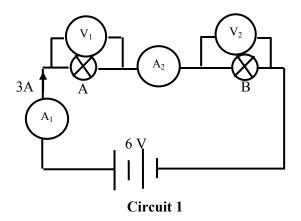
The circuit consisted of two identical dry cells, two identical light bulbs and two ammeters all in series and two voltmeters across each bulb. Ammeters and voltmeters were labelled  $A_1$ ,  $A_2$ ,  $V_1$  and  $V_2$ , respectively. The light bulbs were labelled A and B as shown in circuit 1. The total current and voltage of the circuit were presented as 3A and 6V respectively.
