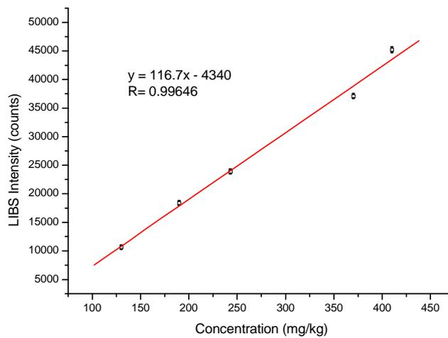
**Figure 3.** Calibration curve for Cr I 425.433 nm line.
