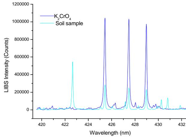
**Figure 2.** LIBS spectra of  $K_2CrO_4$  and Soil sample.
