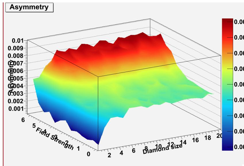
**Figure 2.** Asymmetry of the positrons originating from the diamond. Again, there are statistical fluctuations in the data.
