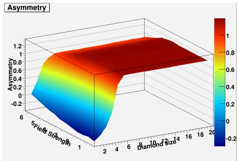
**Figure 4.** False asymmetry due to the positrons originating from the beam stop.
