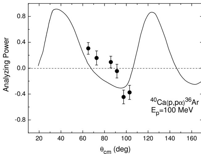
Figure 2: Analyzing power distribution for the reaction  $^{40}\text{Ca}(p,p\alpha)^{36}\text{Ar}$  at an incident energy of 100 MeV. Also see caption to figure 1 for further details. The curve is a prediction of the DWIA as described in the text.
