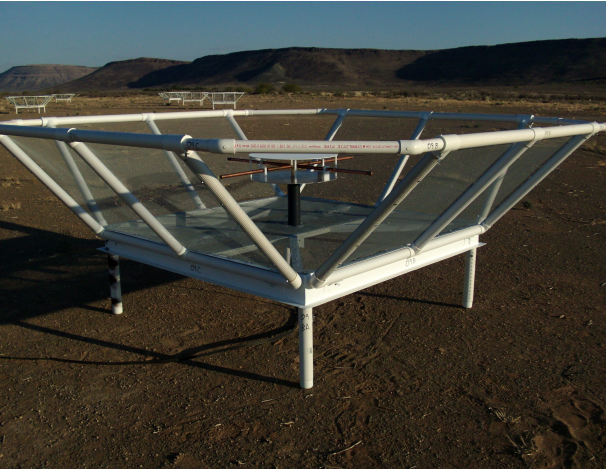
Figure: A PAPER dipole
