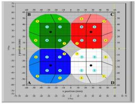
**Figure 1.** Schematic diagram of the HPGe crystals of the iThemba LABS segmented clover detector. The four crystals are labelled as A, B, C, D.
