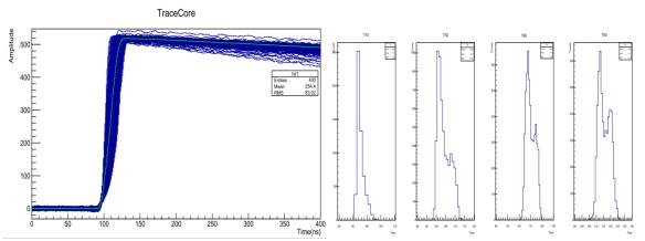
**Figure 2.** Left: The average (green line) and the individual (blue lines) traces for interaction 1, position (-5, 27), which is near the surface of crystal B. Right: The measured individual rise times for each trace for position 1.
