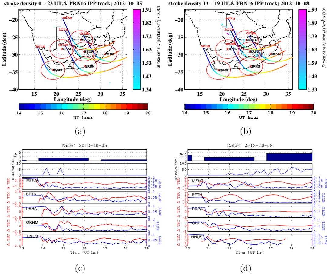
Figure 2: Top rows:corresponding TEC measurement paths (IPP at 350 km) from PRN 16 between 13:00 and 19:00 UT on (a) 5 October, 2012 and (b) 8 October, 2012. Bottom row: Bottom rows: Kp index, stroke rate, STEC variations ( $\Delta$ TEC) and ROTI for PRN 16 on (c) 5 October, 2012 and (d) 8 October, 2012
