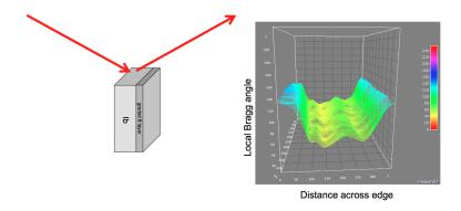
**Figure 4.** A plane wave monochromatic dispersive case topograph at just a single point on the flank of the rocking curve is presented with a view of the sample edge.
