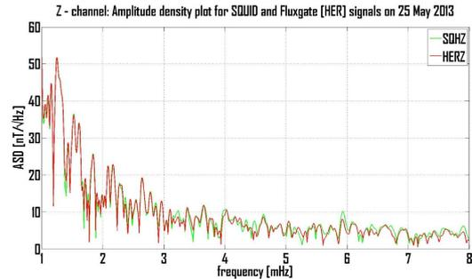
**Figure 4.** SQUID and Fluxgate  $z$ -channels spectra compared to check for correlation of frequency components contained in fluxgate and SQUID data-sets.
