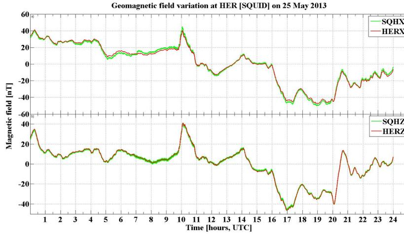
**Figure 2.** SQUID  $x$  (SQHX) and  $z$  (SQHZ) channels, plotted with their corresponding fluxgate  $x$  (HERX) and  $z$  (HERZ) channels for calculation of the correlation of SQUID and fluxgate data-sets in the time domain.
