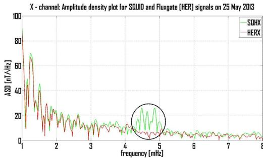
**Figure 3.** SQUID and Fluxgate  $x$ -channels spectra compared to check for correlation of frequency components contained in fluxgate and SQUID data-sets.
