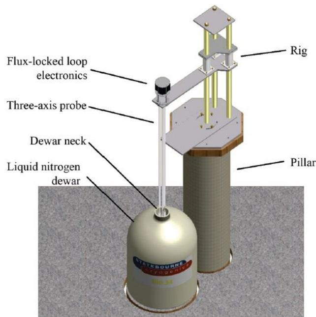
**Figure 1.** Schematic of SQUID dewar and rig (Image: courtesy of [7] )
