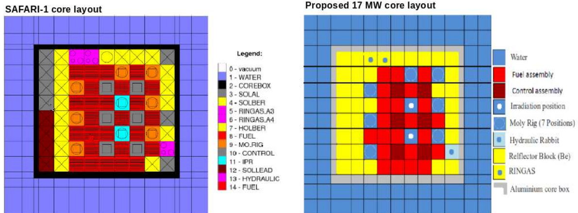
Figure 2. The Proposed 17 MW core layouts
