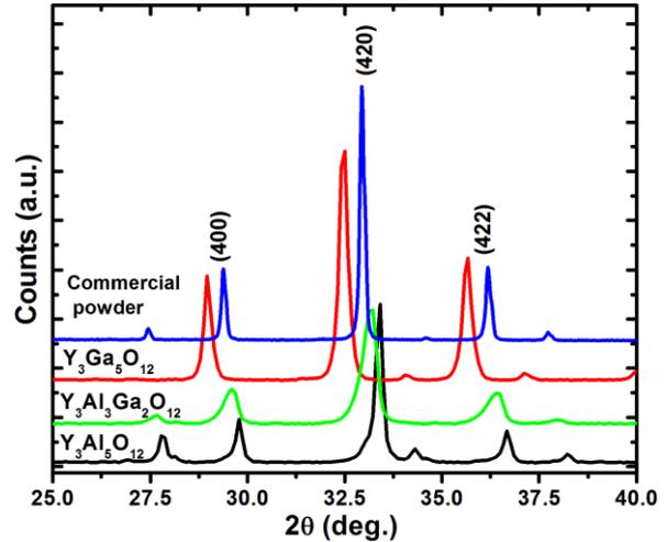
**Figure 1 (b)** XRD patterns of the commercial and prepared  $Y_3(Al_x,Ga_y)O_{12}:Tb$  powder, showing the change in the peak position with different Ga concentrations.
