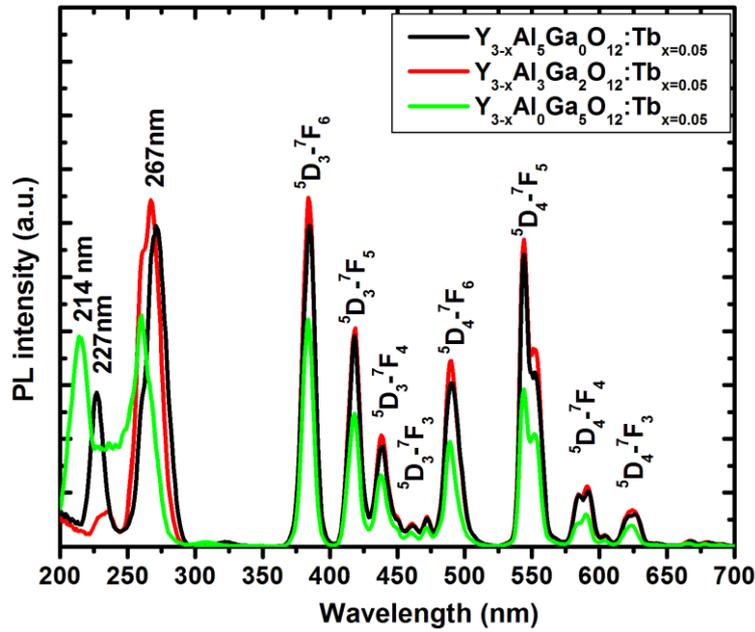
**Figure 4** PL excitation and emission of the prepared  $Y_{3-x}(Al_xGa_{5-x})_5O_{12}:Tb_{x=0.05}$  powder with different Ga concentration.
