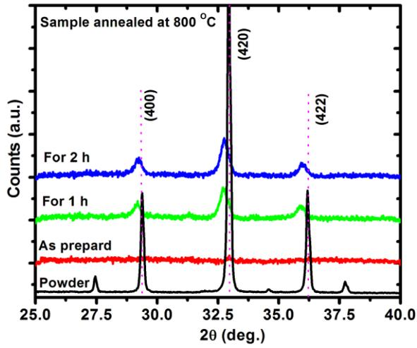
**Figure 1 (a)** XRD patterns of the  $Y_3(Al,Ga)_5O_{12}:Tb$  phosphor powder, and  $Y_3(Al,Ga)_5O_{12}:Tb$  films as prepared and annealed at  $800\text{ }^\circ\text{C}$ .
