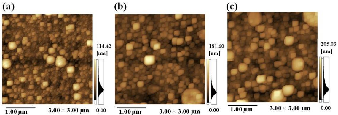
**Figure 3** AFM images of the surface of the  $Y_3(Al,Ga)_5O_{12}:Tb$  films (a) as prepared and annealed at  $800\text{ }^\circ\text{C}$  for (b) 1 h and (c) 2 h.
