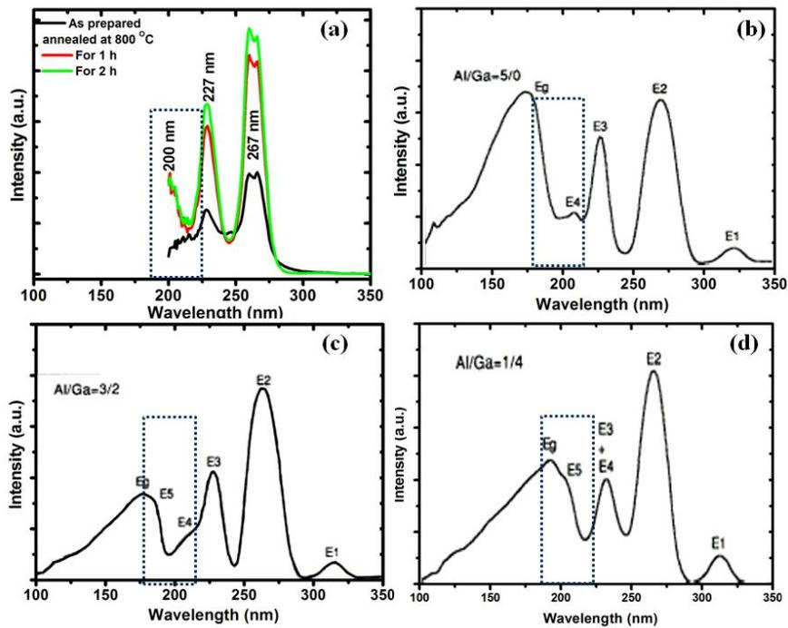
**Figure 4 (a)** PL excitation of the  $Y_3(Al, Ga)_5O_{12}:Tb$  films as prepared and annealed at  $800\text{ }^\circ\text{C}$  for 1 h and 2 h. **(b)-(d)** PL excitation of the  $Y_3(Al, Ga)_5O_{12}:Tb$  powder with different Ga concentration.
