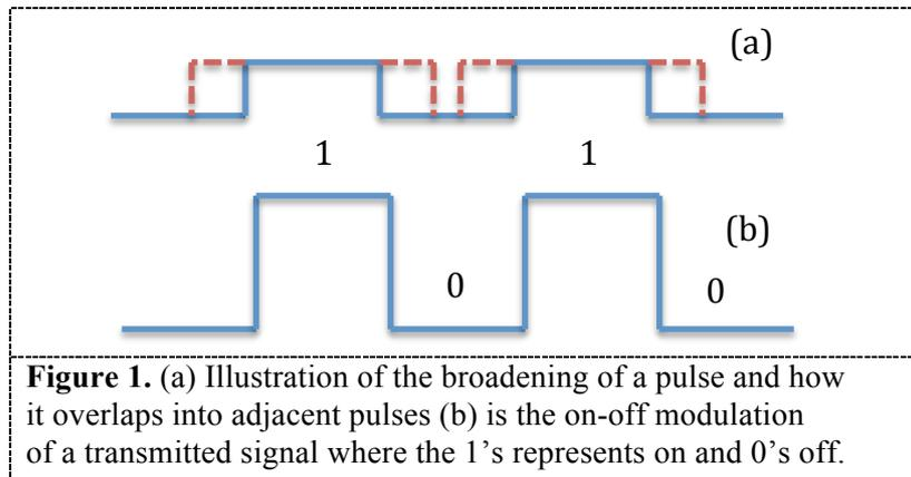
**Figure 1.** (a) Illustration of the broadening of a pulse and how it overlaps into adjacent pulses (b) is the on-off modulation of a transmitted signal where the 1's represents on and 0's off.
