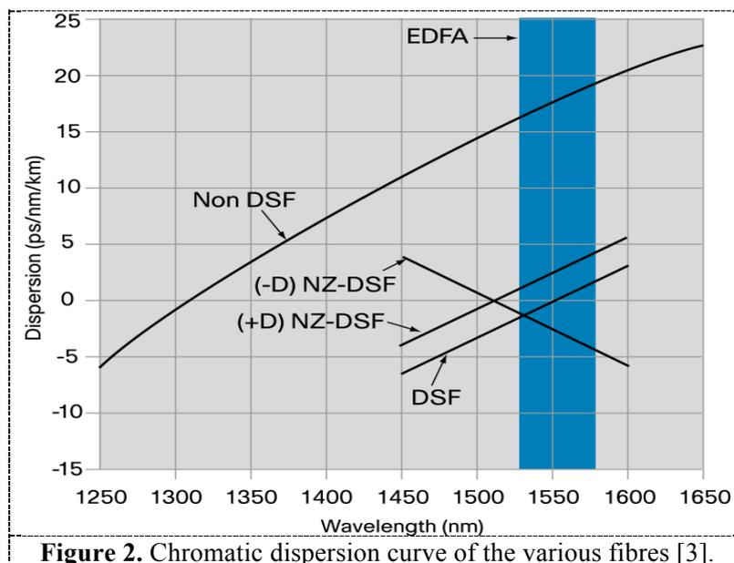
**Figure 2.** Chromatic dispersion curve of the various fibres [3].
