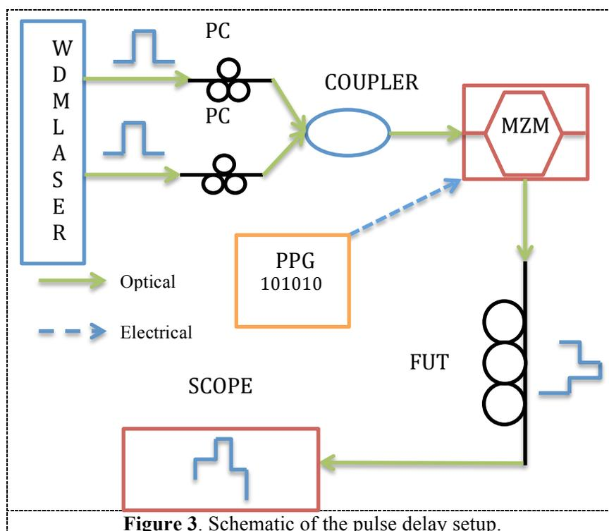
**Figure 3.** Schematic of the pulse delay setup.
