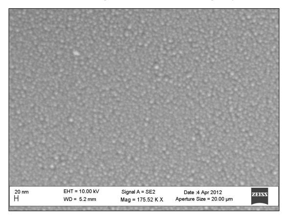
**Figure 1**: An SEM image of Ge nanowires deposited using Ag as a catalyst. It is seen from the image that the wires have very small diameters and that they are oriented vertically on the substrate.
