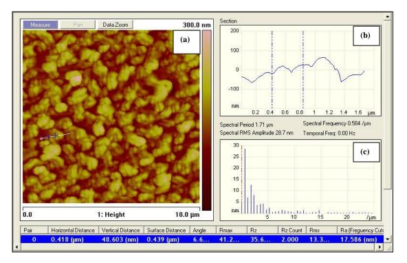
**Figure 2**: (a) Top view of an AFM image obtained from samples where Ag was used as a catalyst. Ge was deposited for 12 minutes using RF magnetron sputtering at a power of 130 W. The chamber pressure was kept at 3x10-3 Torr. (b) and (c) Measurements on the sample surface (see mark on image) showed that the vertical height of the chosen peak is 48.6 nm and surface (area) roughness is approximately 17.6 nm.
