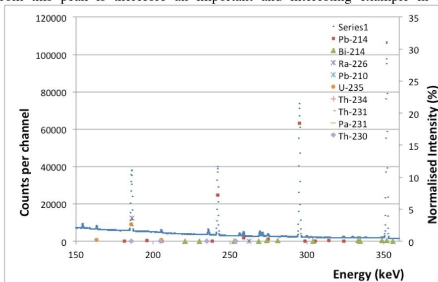
Figure 1: Energy region from 150 - 360 keV from gamma-ray spectrum from reference material (IAEA U) containing uranium in equilibrium with its daughters. The relative intensities of the principal gamma transitions are also shown
