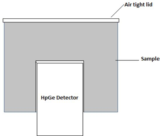
Figure 2: Schematic of the counting geometry with the sample in a Marinelli beaker
