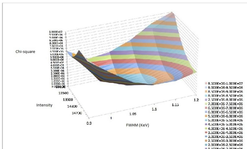
Figure 4. Chi-squared surface for co-axial detector illustrating how the surface varies with changes in the FWHM and the intensity of the <sup>235</sup>U peak. The value of the intensity at the minimum is a sensitive function of the value of the FWHM.
