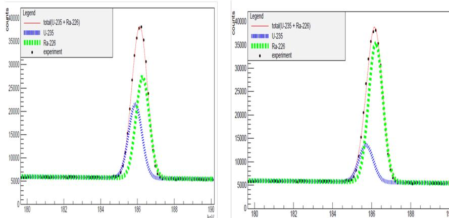
Figure 3. Data points together with fit of two Gaussians plus background using ROOT. Sample IAEAU reference material in equilibrium; detector: BEGe. (a) With a calibration slope of 0.12553 keV per channel and (b) with a calibration slope of 0.12531 keV per channel; FWHM 0.85 keV in both cases.
