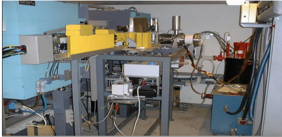
Aarhus microtron injector showing the electron gun
