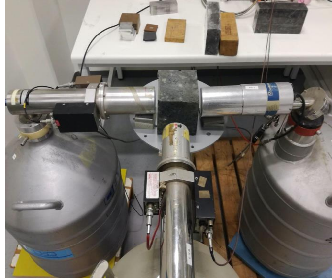
K6 rock in between HPGe detectors
