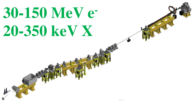
Fig.2 – STAR machine as an example of Paradigm A. Overall length about 12 m.
