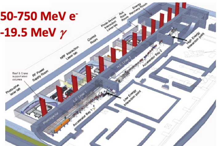
Fig. 197. Isometric 3D view of Building Layout of the Accelerator Hall & Experimental Areas
