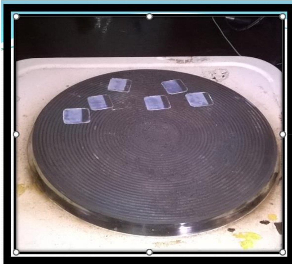
FTO glass with \text{TiO}_2 deposited on and annealing at 500\text{ }^\circ\text{C} in air
