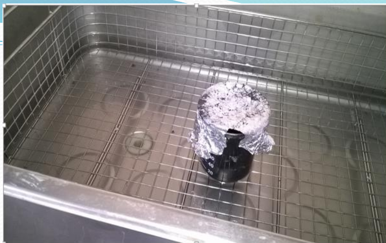
(b) Sonicate for 3 hours at 45 °C temperature to enhance metal dispersion
