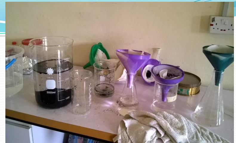
(c) Washing with distilled water to a pH of 7
