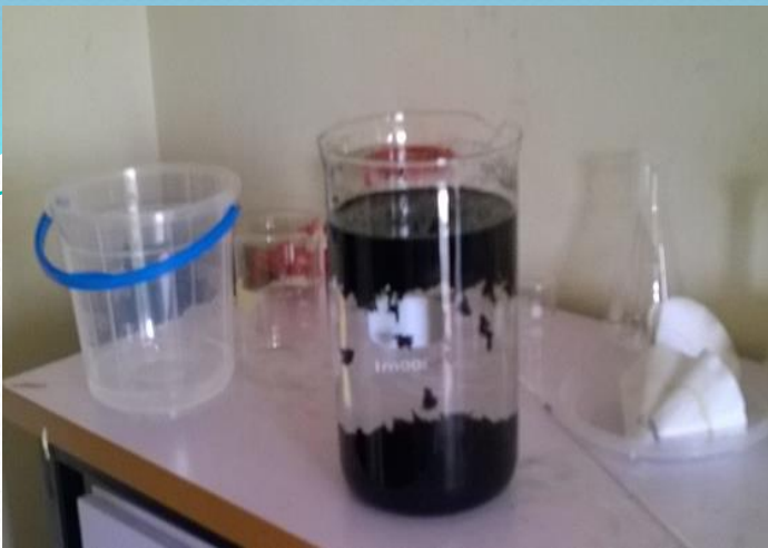
(a) CNTs + acid in ratio 3: 1 ( \text{H}_2\text{SO}_4 : \text{HNO}_3 ) to remove metallic impurities
