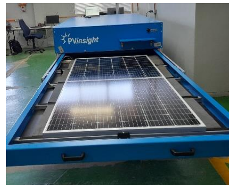
Fig. 4: The solar simulator used for indoor characterization of bPV module, with a module loaded and ready to be tested.
