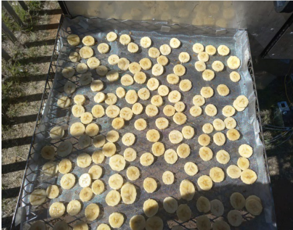
Fig. 4. The loaded tray with banana slices with a 1 mm wire mesh that was placed on top of the drying tray during a drying experiment.
