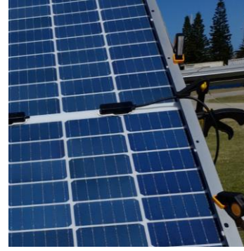
Fig. 6: Challenge of module self-shading when characterizing the rear surface due to the module frame and module cables.
