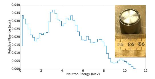
Neutron beams produced with HDPE collimator (Ø 0.8 cm)
