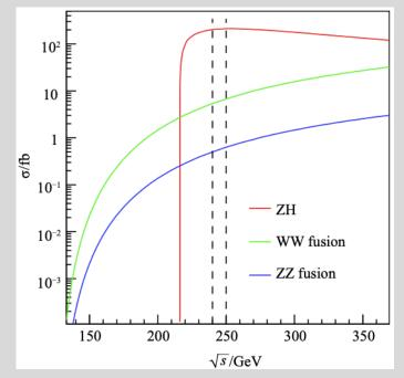
• Production cross sections of the Higgsstrahlung, WW – fusion and ZZ – fusion processes as functions of center-of-mass energy,  $\sqrt{s}$ .
