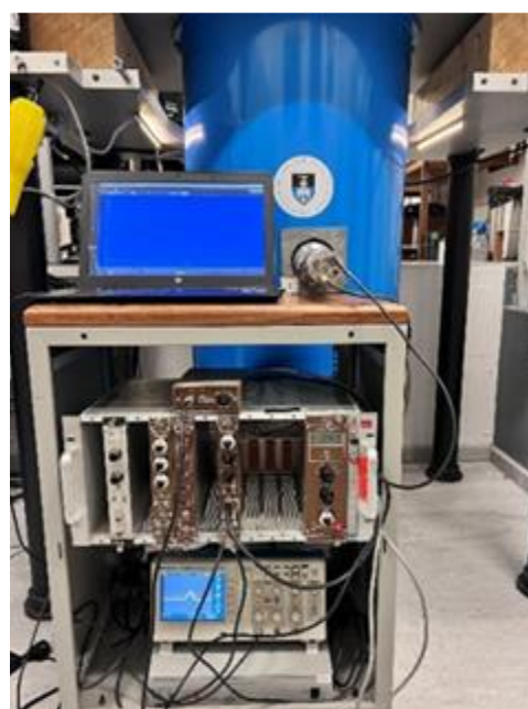
Figure 3. The NaI scintillation detector positioned at a 0° angle from the ^{60}\text{CoCo}(\text{hcp}) crystal.
