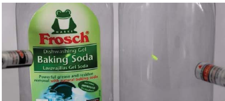
Fig. 1: Application of up-conversion based luminescent markers on labels (left bottle) and in the packaging material (right bottle) [2].
