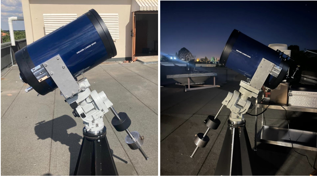
Figure 2. The full operating telescope with counterweights, properly aligned and well-balanced.
