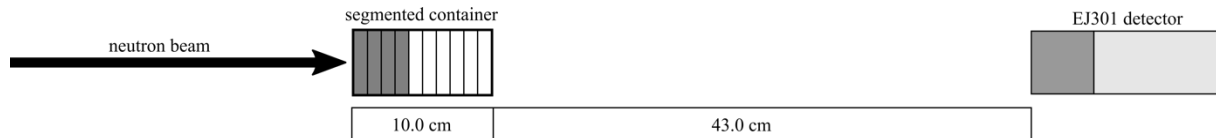
Figure 1. Fast neutron transmission experimental set-up. A pencil beam of ^{241}\text{Am-}^9\text{Be} neutrons is incident on the segmented container, where the shaded sections correspond to a measurement of 4.0 cm sample thickness. Transmitted neutrons are incident on a 2'' x 2'' EJ301 organic liquid scintillator detector.
