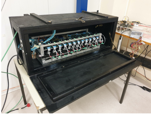
Figure 2: Light tight box for the phase-2 PMT teststand showing 12 PMT-Blocks on the tray.
