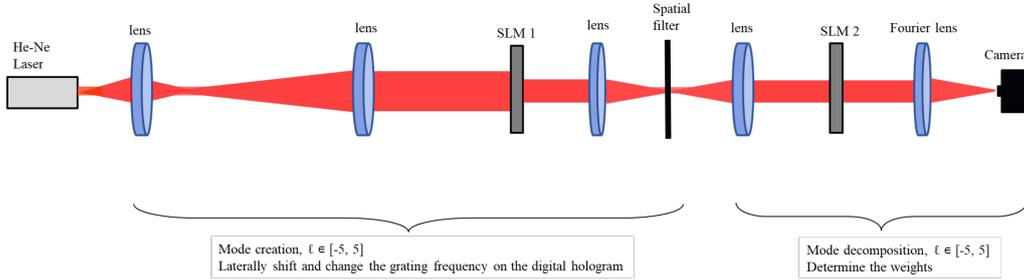
Figure 3: Schematic experimental setup: Lens before SLM 1 enlarges the beam. The first SLM is illuminated with horizontally polarized light and encoded with holograms that perform complex amplitude modulation and impose tilt angle and lateral displacement. An incoming LG mode from SLM 1 selected by the spatial filter is modally decomposed by the second SLM addressed by detecting hologram. At the Fourier plane the on-axis intensity is detected by the camera.
