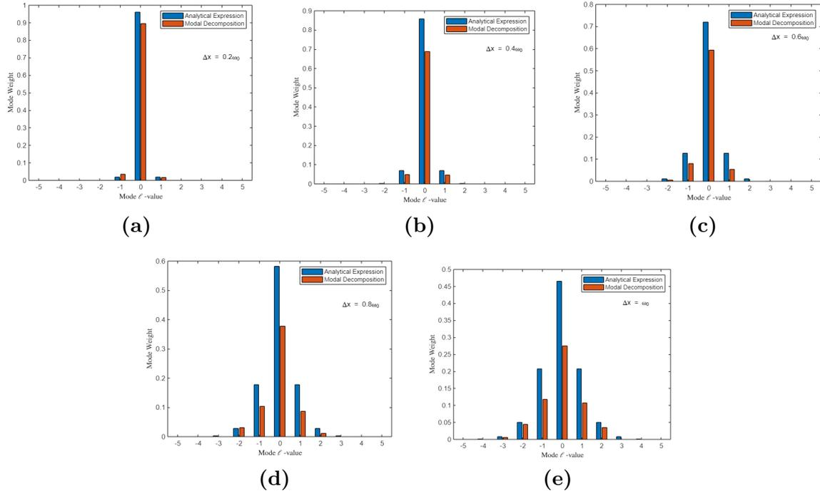
Figure 6: A case when lateral displacement imposed was increased. A mode index value,  $\ell = 0$  of beam waist,  $\omega_0 = 0.35\text{mm}$  was the input mode. (a)-(b) shows the spectrum obtained from the experimental setup and crosstalk analytical expression for the same amount of lateral displacement.
