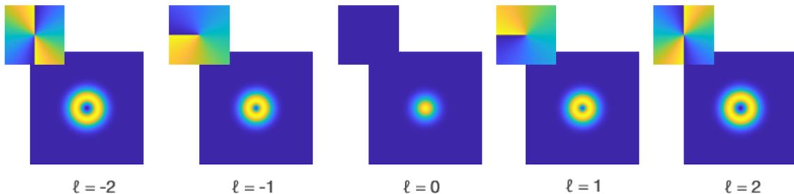
Figure 1: Intensity and phase (top left corner) of OAM beams with  $\ell = 2$  to  $-2$ .
