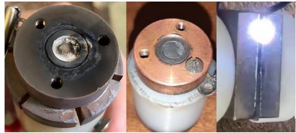
**Figure 2.** The three VATs used in this work. Left to right: Bismuth coaxial thruster showing clear cathode erosion, coaxial steel thruster with minor erosion and planar steel thruster during arc operation.
