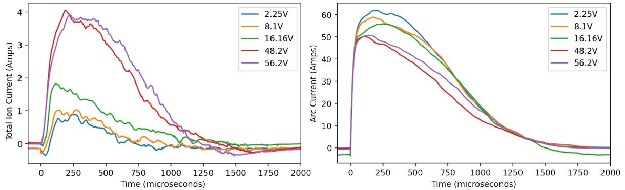
**Figure 5.** Planar steel thruster ion and arc currents over the range of ion collector negative bias voltages tested.
