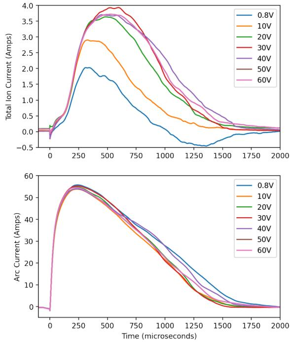
**Figure 3.** Coaxial bismuth thruster ion and arc currents over the range of ion collector negative bias voltages tested.
