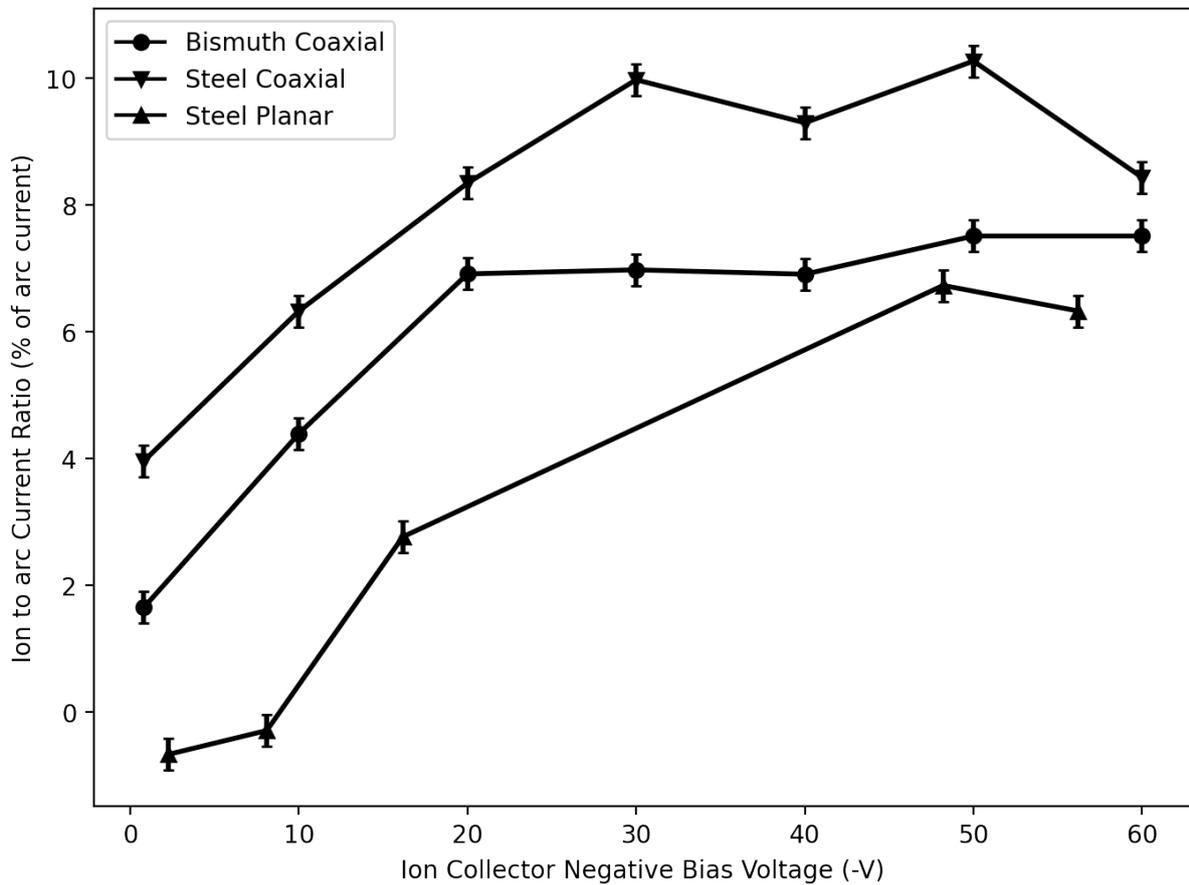
**Figure 6.** Ion to arc current ratio versus ion collector negative bias voltage, expressed as a percentage of the arc current.
