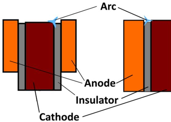
**Figure 1.** Cross section showing the simple geometry of coaxial (left) and planar (right) thrusters.
