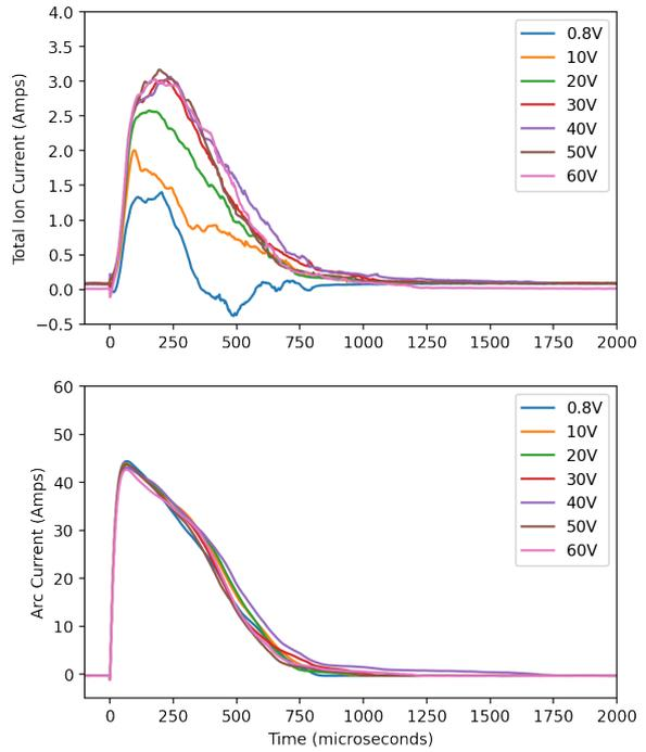
**Figure 4.** Coaxial steel thruster ion and arc currents over the range of ion collector negative bias voltages tested.
