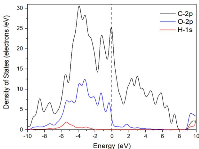
**Figure 3.** Density of states for GQDs calculated from material studios DFTB+ Energy module. The atoms and their highest occupied states are shown with their orbitals.
