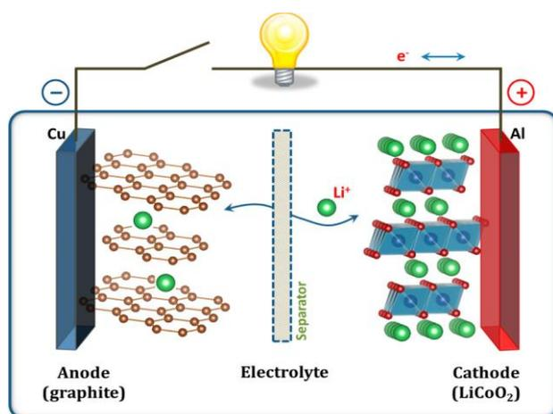
**Figure 1.** Working principle of LI batteries [7]. The anode material used is graphite.
