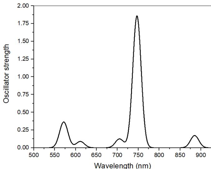
**Figure 4.** UV-vis spectrum of GQDs. It shows the wavelengths of UV or visible light that are absorbed or transmitted through the material of interest. The highest peak is located at 750 nm of wavelength with two located at 575 and 885 nm.
