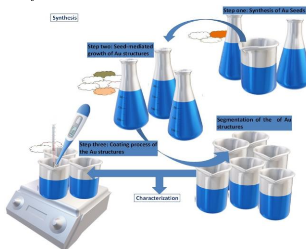
Figure 2-1: Synthetic experimental setup for synthesis of Au@SnO 2 nanocomposite structures.
