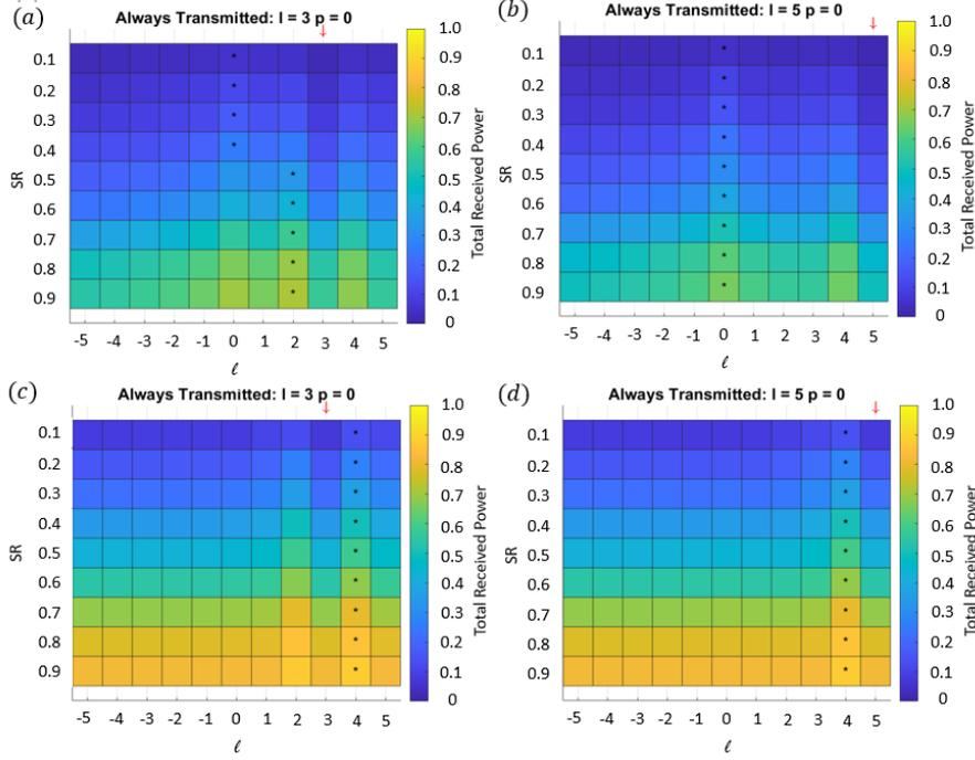
**Figure 2.** Total powers received when a single OAM beam is transmitted and combined with other beams. The mode combined with the transmitted mode which provides the largest received power is shown with an asterisk. In (a) and (c) the transmitted mode is  $\ell = 3$  and has a lower  $M^2$  whereas in (b) and (d) the transmitted mode is  $\ell = 5$  and has a higher  $M^2$ . (a) and (b) show results for un-normalised beams whereas (c) and (d) show results for normalised beams.
