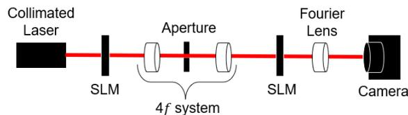
**Figure 1.** Experimental setup that is analogous to the simulation method used (SLM: Spatial Light Modulator)
