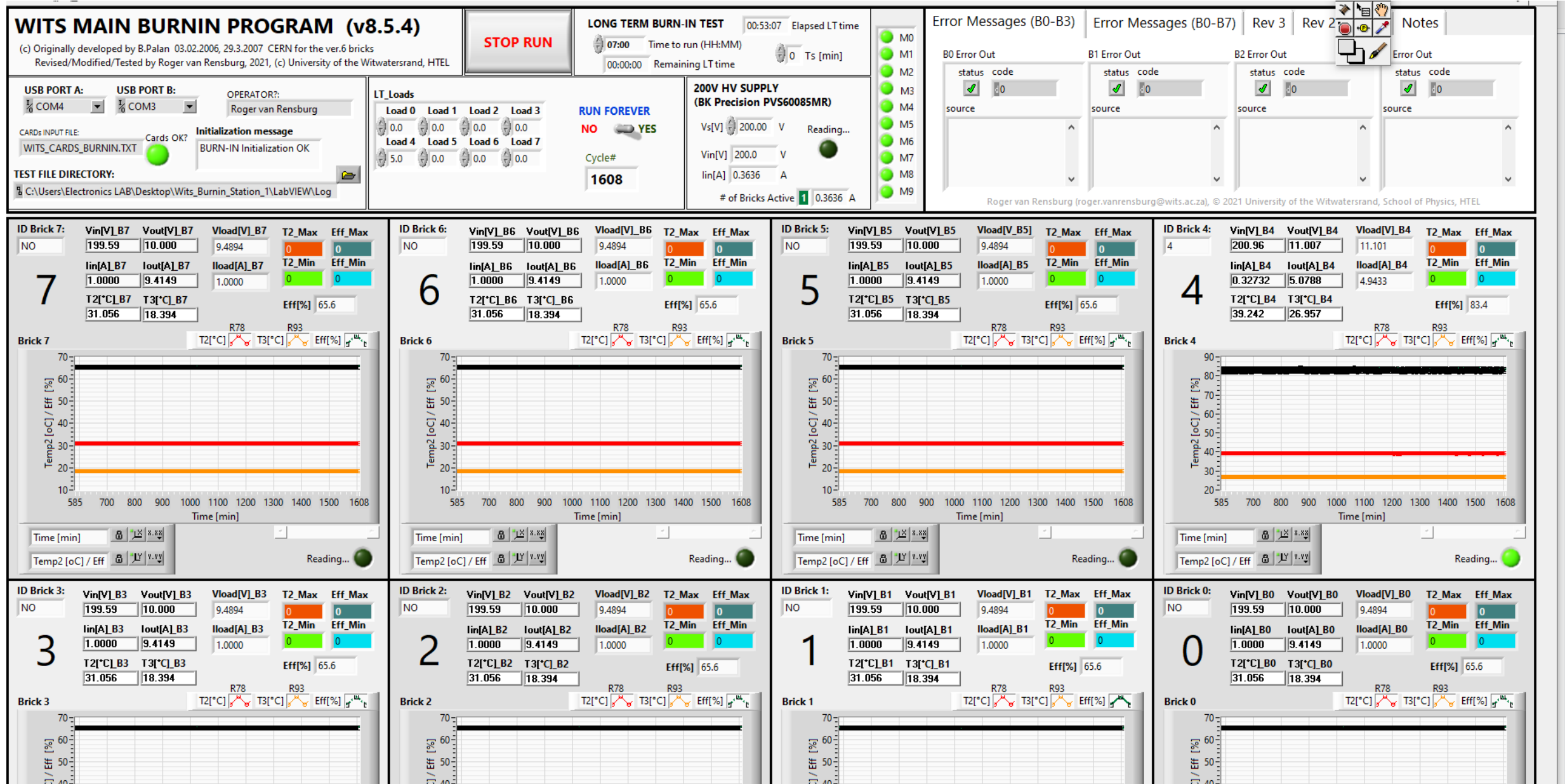
Fig.22 The Burn-in Test-Station LabVIEW GUI
